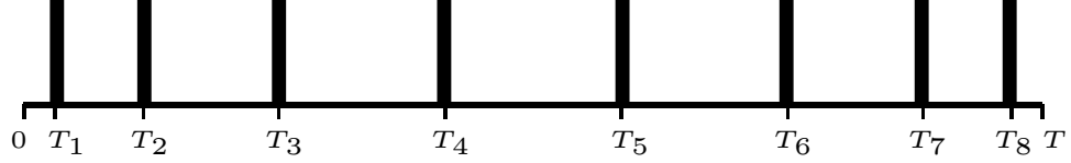
Figure 1.11: Pulse sequence for UDD sequence for a cycle time of T and the number of \pi pulses in one cycle of sequence is eight. Filled bars represent \pi rotation pulses.
