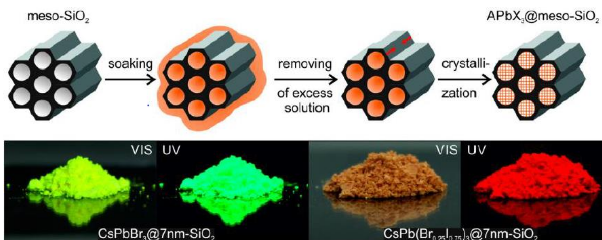
Fig4: Schematic of the template-assisted synthesis of APbX 3 NC in mesoporous silica and images of perovskite solution impregnated mesoporous silica in daylight and under UV illumination (Taken from Ref 20)
