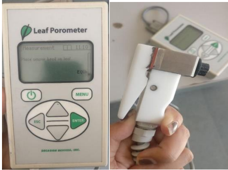
Photo 5: Leaf Porometer Controller (left) and Sensor Head (right), photo taken by me
