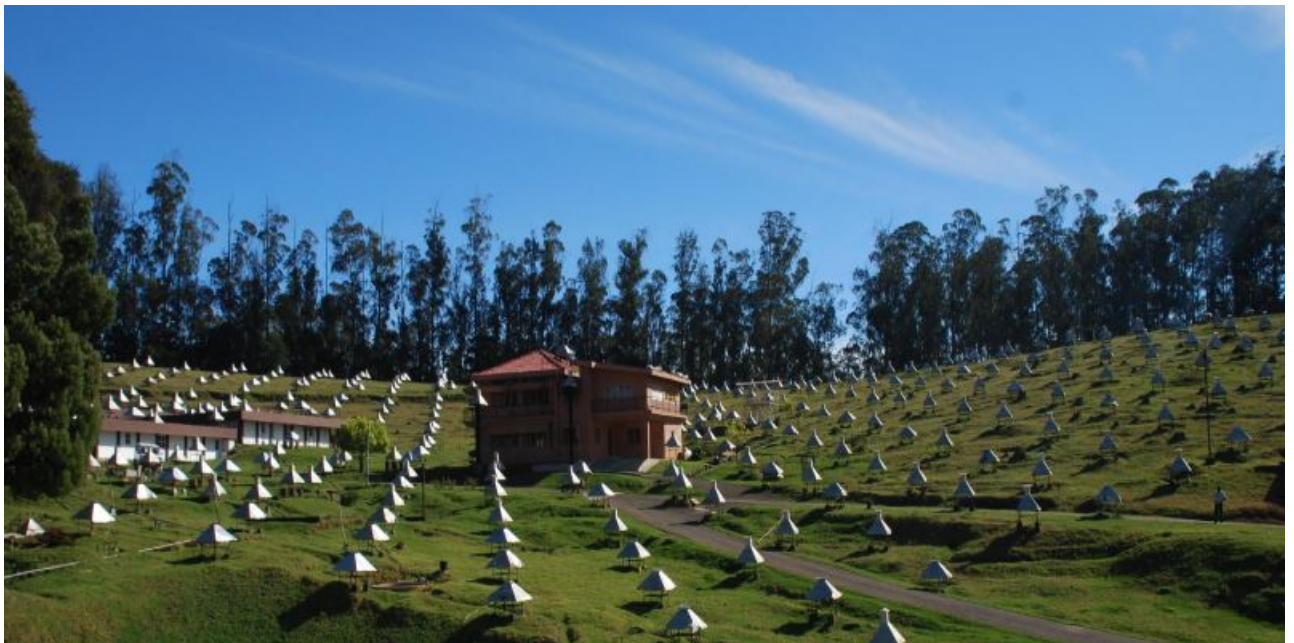
Figure 4.2: Array of air shower detectors at Ooty, India. (Courtesy: GRAPES-3)
