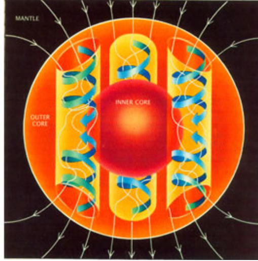
Figure 2.1: Illustration of earth dynamo process, the convection currents lead to circulating electric currents which then generate earth's magnetic field. (Courtesy: Wikipedia.org)
