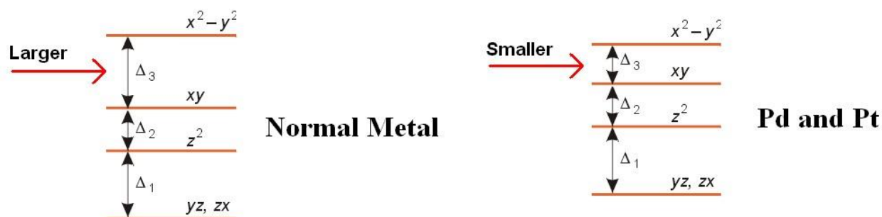
Fig 3. d orbital energy levels of normal metal vs d^8 metals (Source: https://i.imgur.com/53jll.png )
