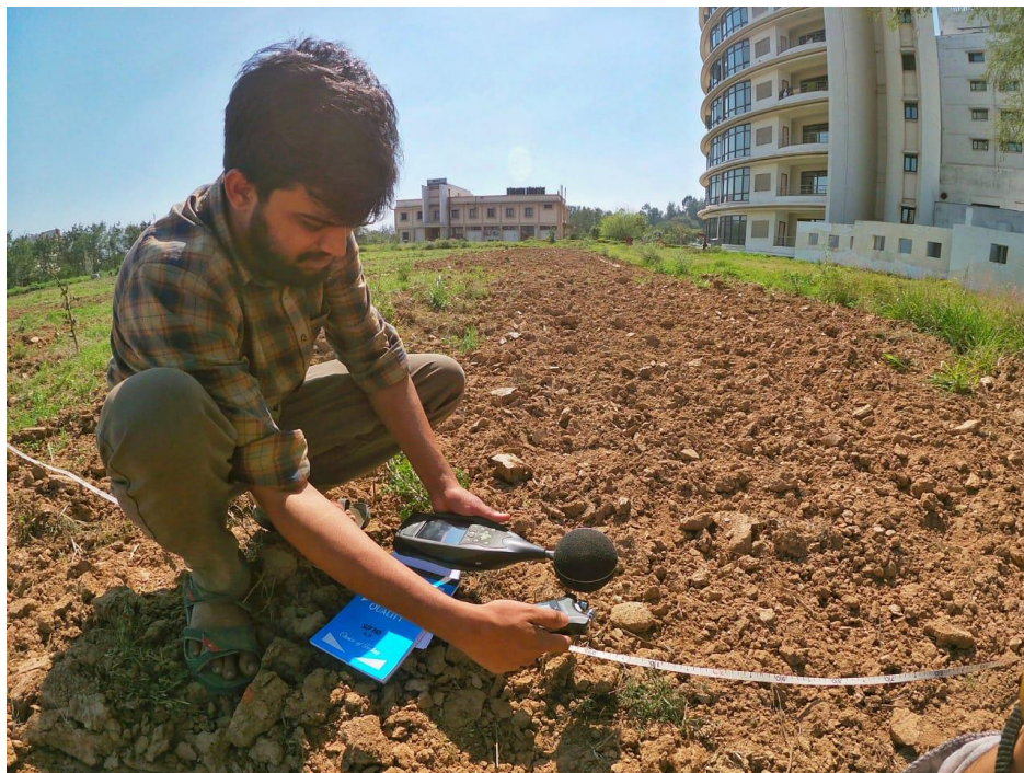
Fig 4.2: measuring SPL during the experiment
