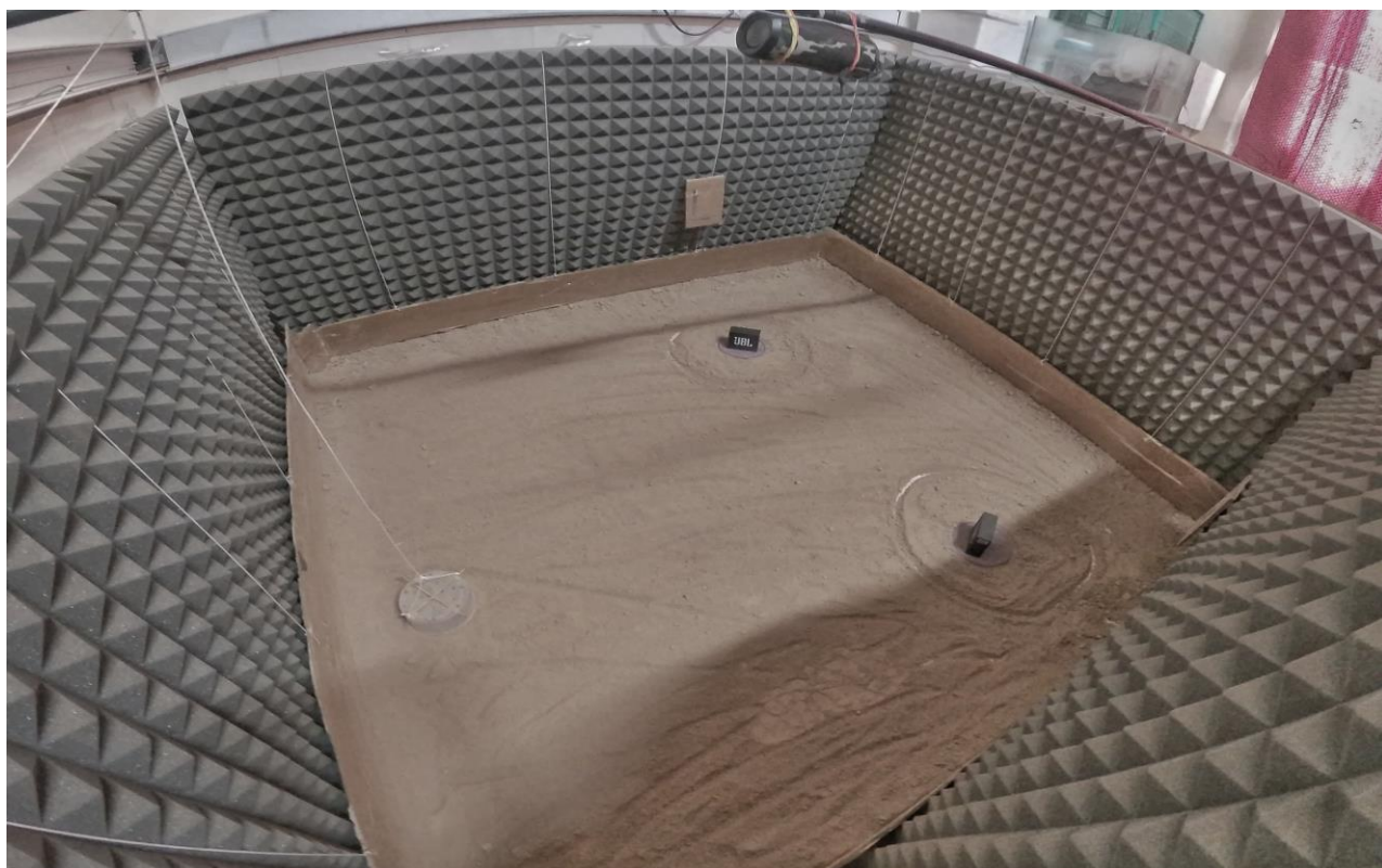
Figure 2.2: Arena for phonotaxis experiment. Two speakers (right) and female releasing point (left) can be seen in the photograph.
