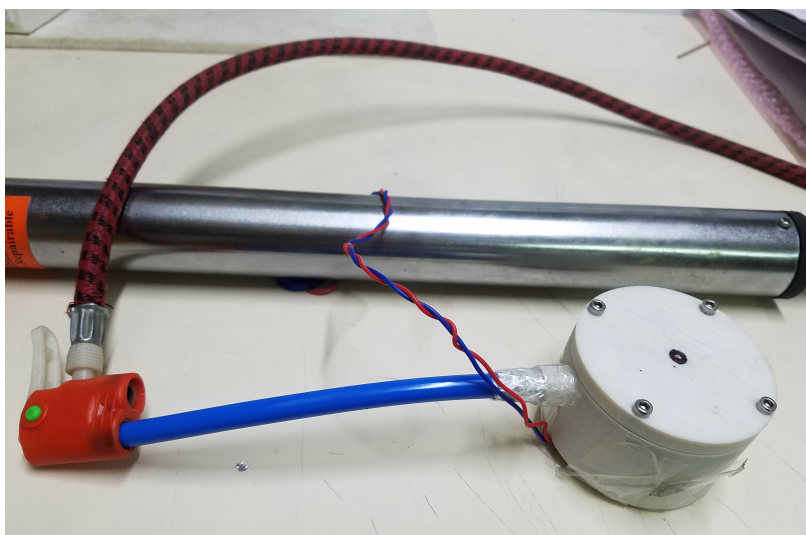
Figure 5.7: Testing leakage with a bicycle pump
