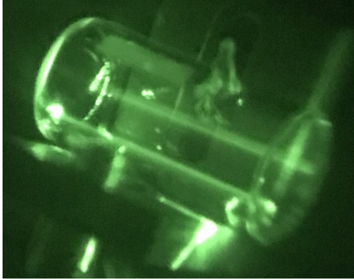
Figure 3.2: Rubidium cell with laser frequency on resonance. Image taken through the IR FindRScope.
