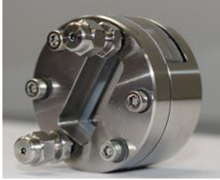
Figure 2.2: Picture of a microfluidic cavity used for VSC. The length of the cavity formed is in the range of 6 – 12 \mu\text{m} .
