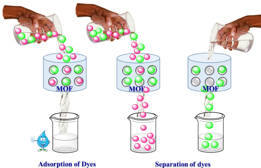
Figure 1.3. Schematic representation showing adsorption and separation of dyes from wastewater by MOF.
