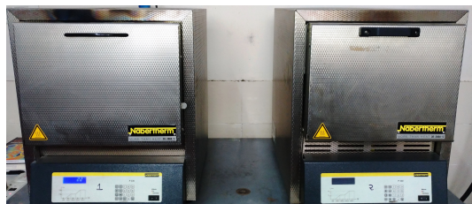
Figure 2.1: Tabletop muffle furnaces used for heat treatments of the samples.
