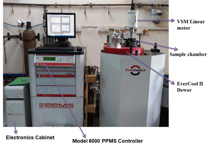
Figure 2.4: 9 T Quantum Design Physical Property Measurement System(PPMS).
