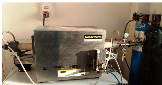
Figure 2.2: Tube furnaces used for heating treatment of the samples in vacuum or argon/ oxygen.
