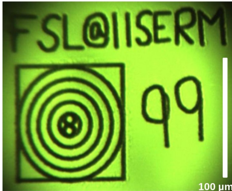
(B) fs laser drawn pattern on glass slide (Objective: 20x, Spot size: 4.4\mu\text{m} , Average power: 3mW, Processing time: 19min 20sec)
