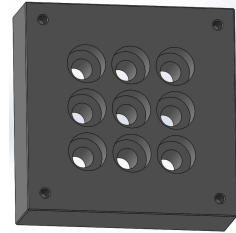
(E) Adaptor for LNR25M/M and Figure 1.2d ( 60 \times 60 \times 18.7 \text{ mm}^3 )
