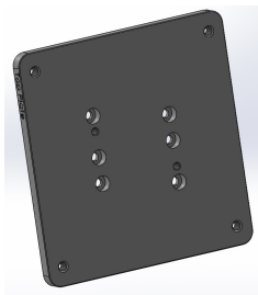
(B) Adaptor for PZT and V-block ( 90 \times 88 \times 5 \text{ mm}^3 )
