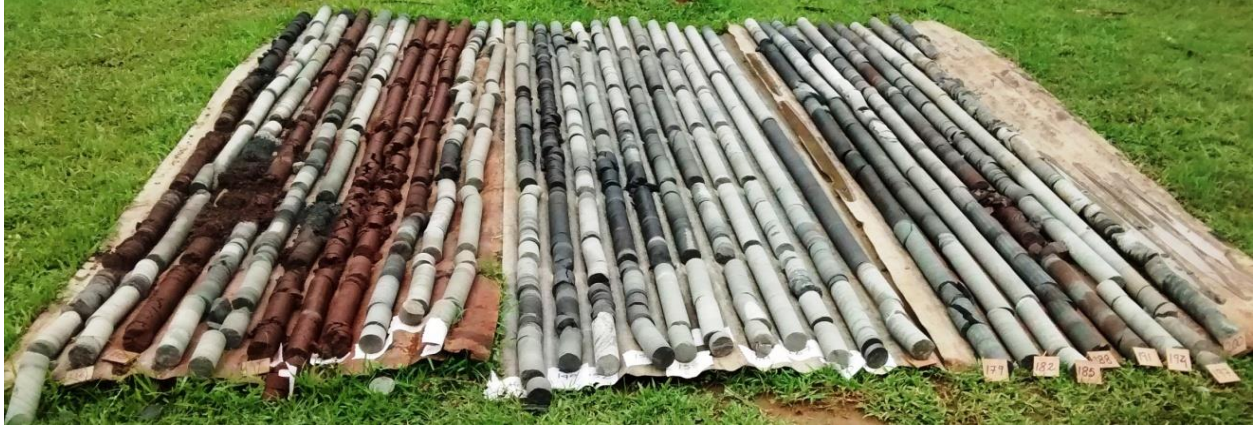
Figure 6: The borehole samples of Panchet and Raniganj Formations, Madhukunda. The retrieved core of 257 meters is placed in order from younger to older (left to right). The younger cores from Triassic are mostly sandstone, shale and mica rich rocks. The Permian rocks in the right comprise of shale, coaly shale and coal as well as sandstone.
