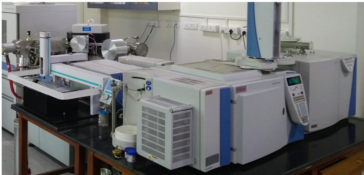
Figure 15: Photograph showing elemental analyzer (EA) coupled with Isotope ratio Mass spectrometer (IRMS).
