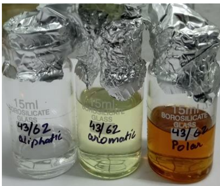
Figure 18: Photograph showing the silica gel column chromatography technique for the separation of different (saturated, aromatic and polar) hydrocarbon fractions.
