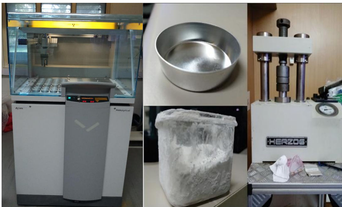
Figure 4.2: XRF Spectrometer at Physical Research Laboratory (PRL), Ahmedabad and Various accessories used for preparing sample pellets.
