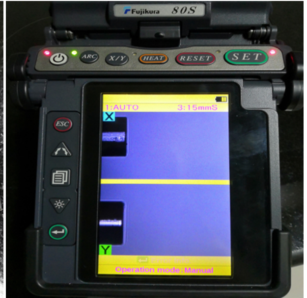
(b) Perpendicular Cut at the end of fiber
