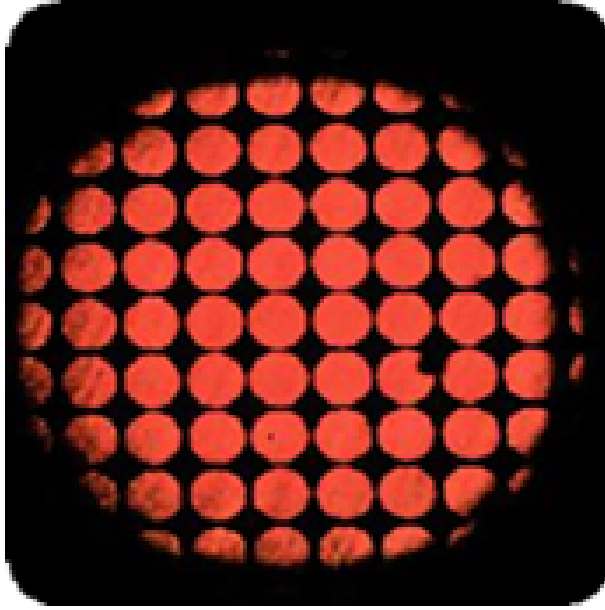
(a) Micro lens array with 10x scan lens
