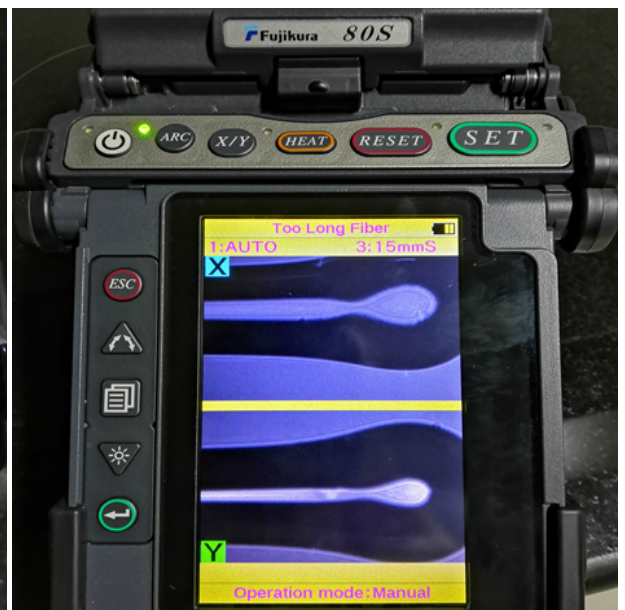
(b) Microsphere in optical fiber
