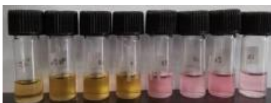
Fig. 2.11 Solutions of m-ADA in THF/water v/v left to right: 90/10, 80/20, 70/30, 60/40, 50/50, 30/70, 20/80, 10/90 showing AIE effect.
