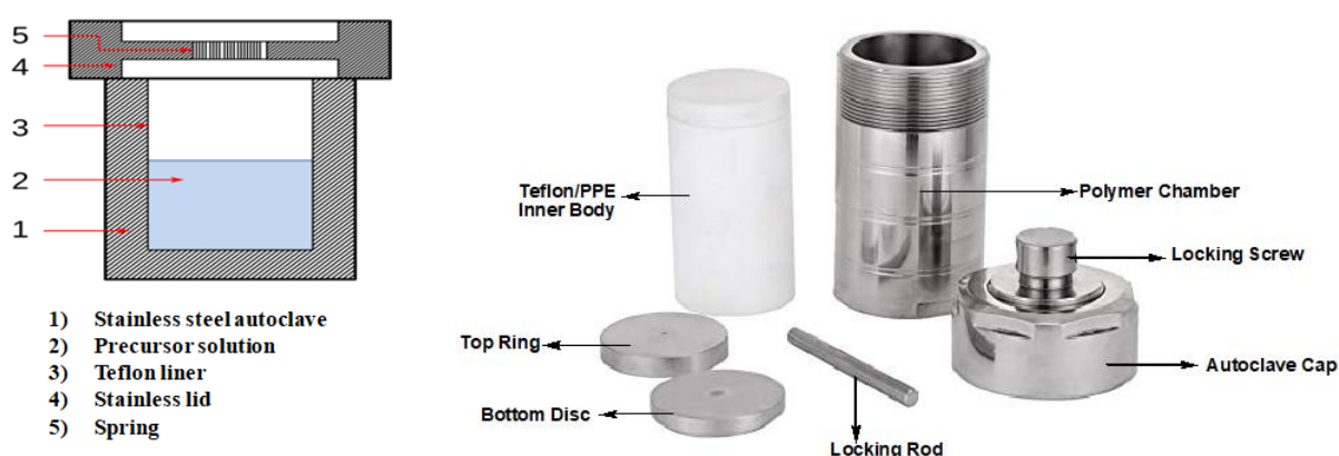
Figure 1.6. Stainless steel teflon reactor for solvothermal/hydrothermal reactions and its schematic diagram.
