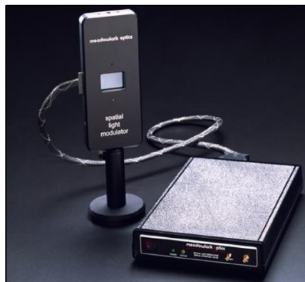
Figure 1.7: LCOS-SLM from Meadowlark optics (Taken from https://www.meadowlark.com/ ).
