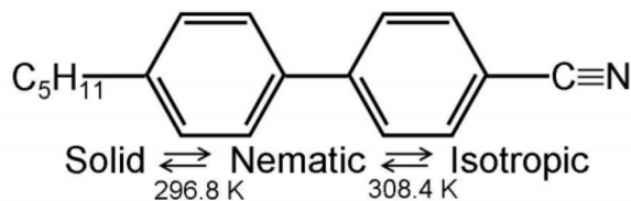
Figure 5.2: Chemical structure of 5CB with its phase transitions
