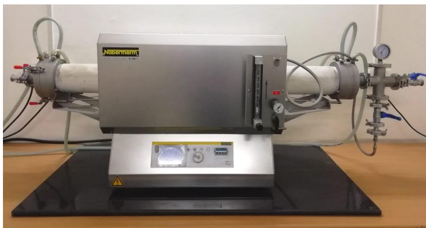
Figure 1.8. Photograph of tube furnace used for pyrolysis.
