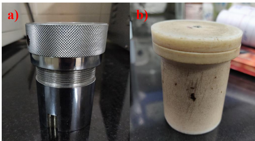
Figure 1.7. a) Steel jacket and b) Teflon reactor used for the Hydrothermal method.
