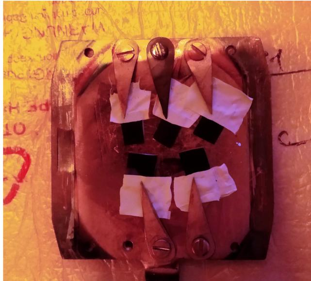
Figure 3.8: Shadow masking with Teflon tape.
