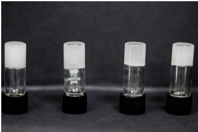
Figure 7. Naming from left:- MBG of water only ( no added pentanol as co-surfactant),MBG of Sucrose 250mM, MBG Sucrose with added pentanol as cosurfactant, MBG of Pentanol only . Each is at W_0 = 100 , 5 min vortexing was done after mixing of all the components, stable gel was formed in each case.
