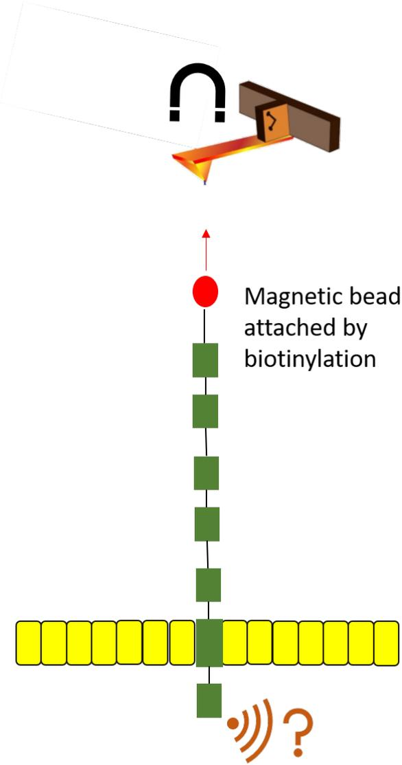
Figure 3.5: Schematic Representation of pulling experiment with magnetic tweezer
