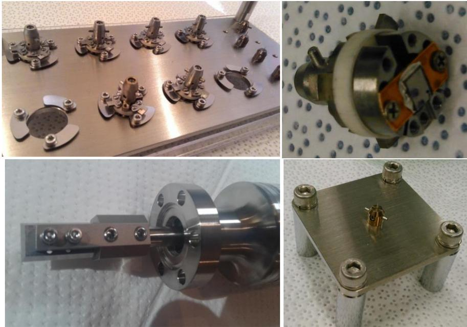
Figure 2.7: (top) Sample holders, (bottom left) image of the UHV cleaver, (bottom right) A tip holder
