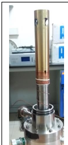
(e): Cryostat with radiation shield
