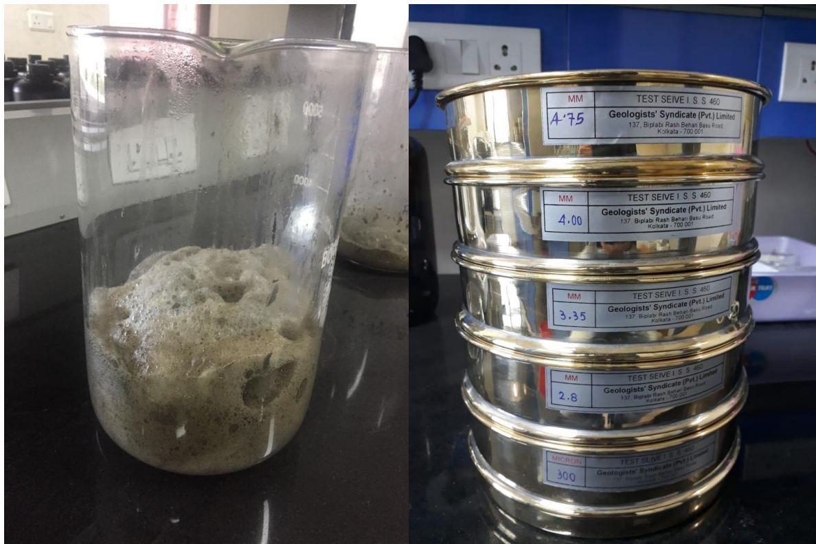
Image5. Wet peroxide oxidation- WPO (Left) and SIEVES set (Right)
