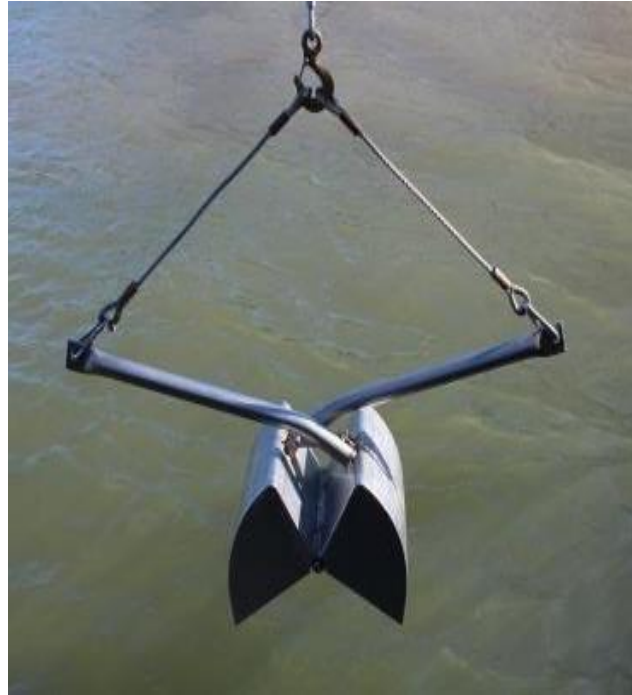
Image1. Van-Veen grab sampler used for surface sediment sampling
