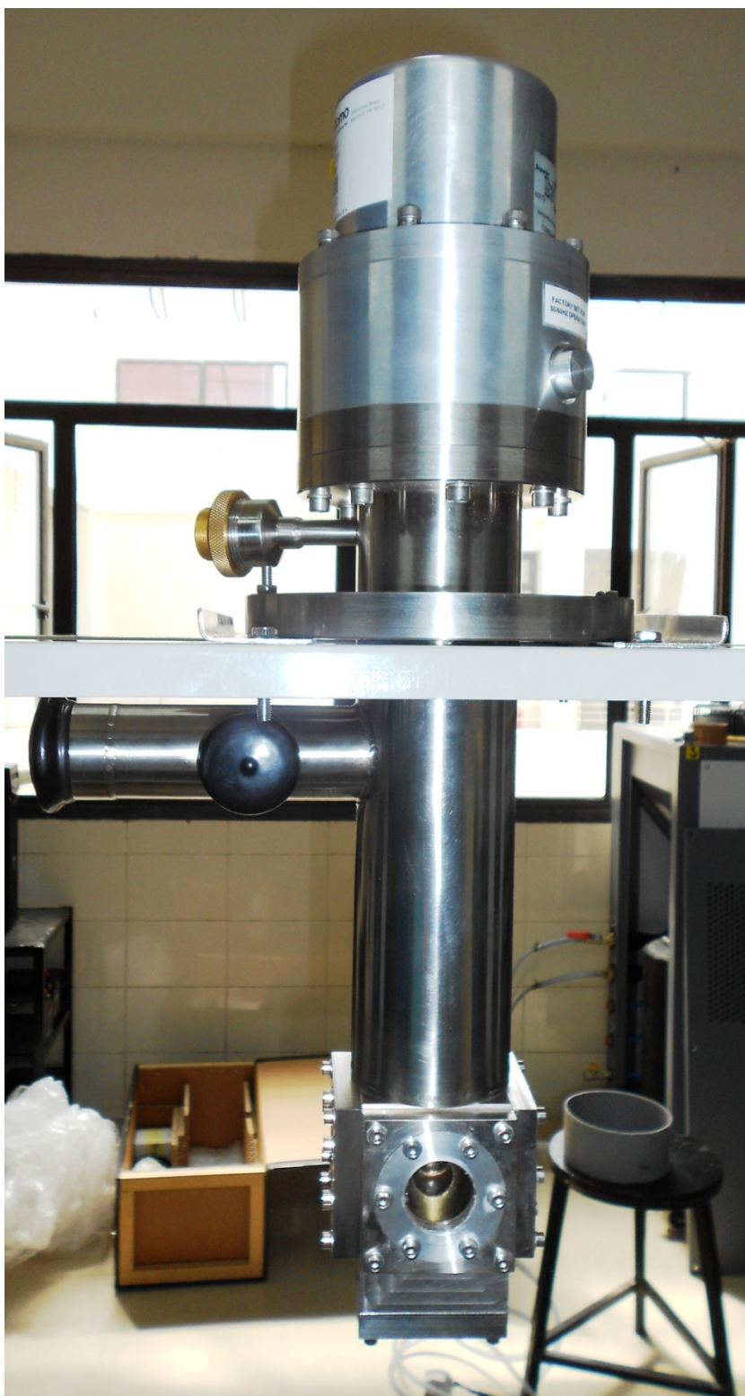
Figure 10: Photograph of the helium compressor cooled cryostat CH-202w/HC4E1 in our experimental set up.
