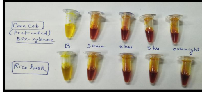
3.5 a): Estimation of hydrolyzed sugar products with BSX XYLANASE using biomass of corncob and rice husk using DNSA method (B represents Blank i.e. without enzyme).
