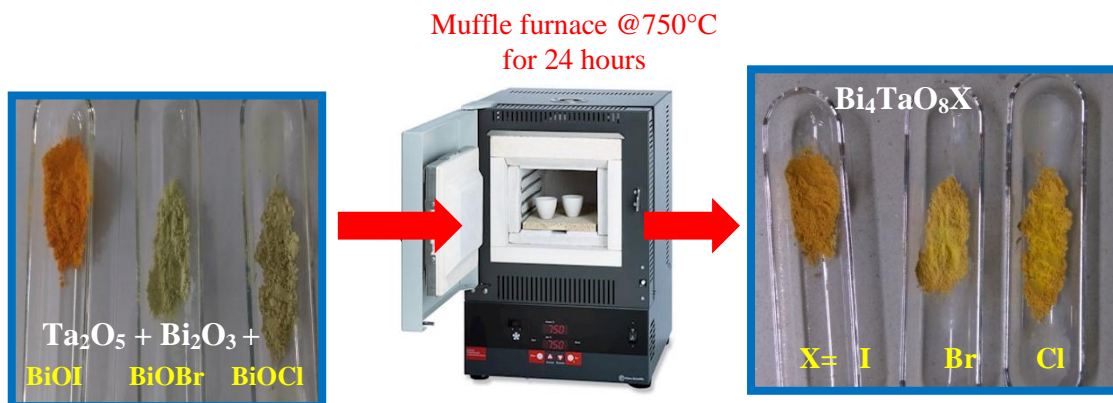
Photo 3.3- Schematic illustration of the synthesis of Bi_4TaO_8X via solid-state route.
