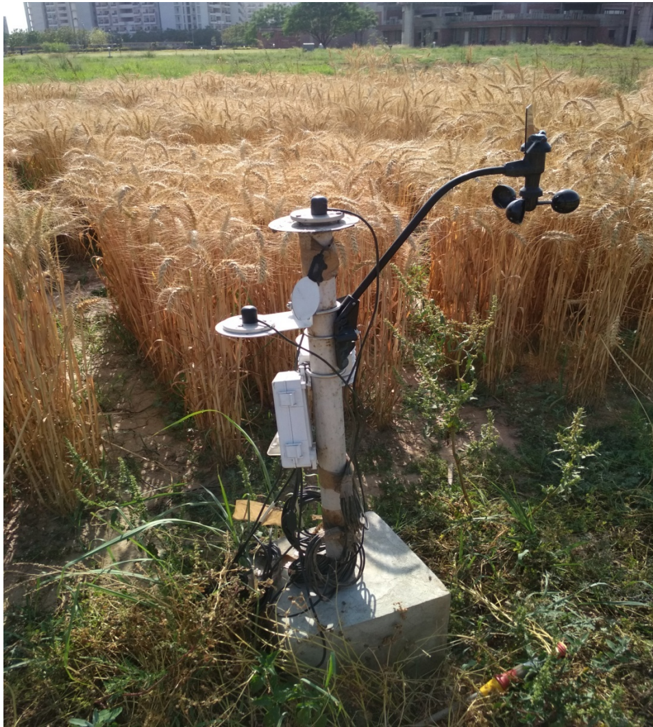
Photograph 2 : The DecagonEM50 device set up in the experimental field.
