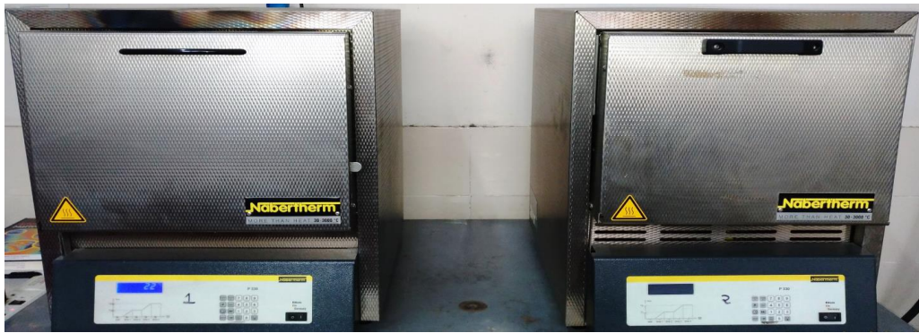
Figure 2.1: Tabletop muffle furnaces used for heat treatments of the samples.
