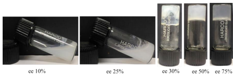
Figure 2.8. Digital images of the precipitates and hydrogels formed by histidine and Zn^{2+} ions with varying ee % of D -histidine. Partial gel formed upon addition of Zn^{2+} ions to a 30% ee solution of D -histidine.
