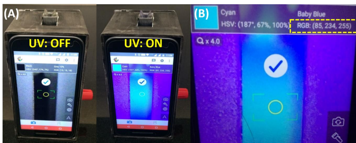
Figure 3-8: (A) Actual photographs of the working of device showing fluorescence signal from Quantum dots. (B) Close-up image of the smartphone application showing the RGB content of the fluorescence from the selected area. The RGB values are marked with a yellow dashed rectangle.
