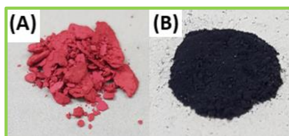
Figure 3.8: Color change: (A) Ni(II)-DMG complex with a red brick appearance and (B) BC-Ni nanorods product after carbonization.
