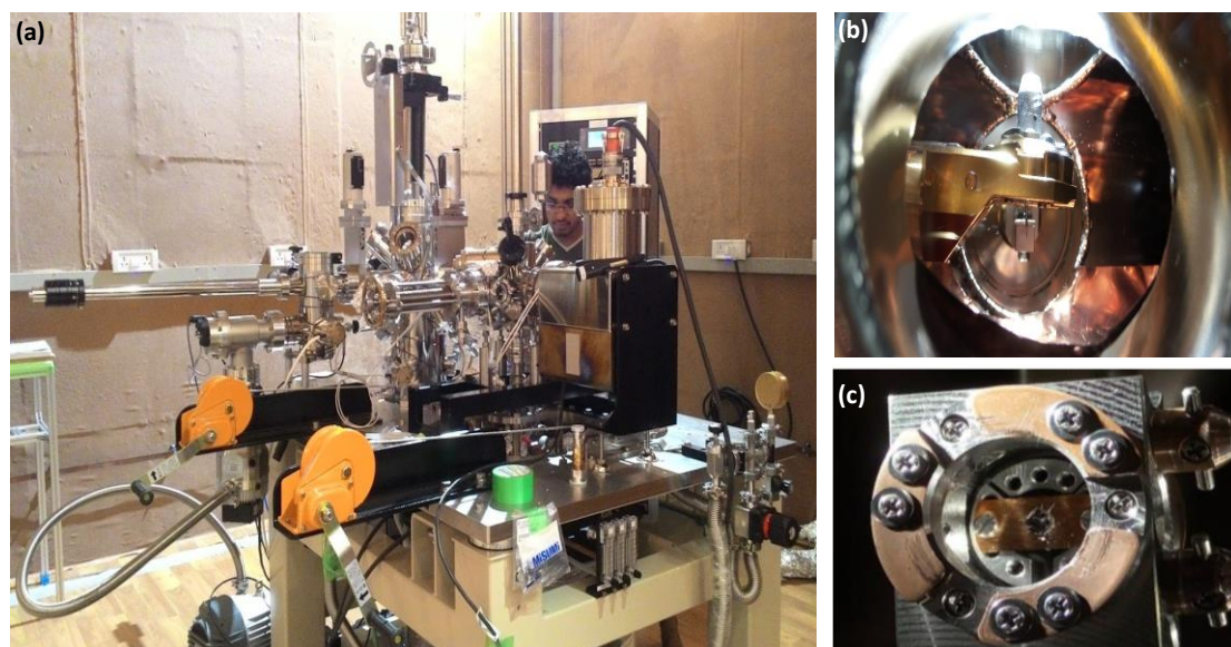
Figure 2.4: (a) A view of STM from a different angle (b) Cleaving stage (c) Cleaved sample tron diffraction (LEED), and an auger electron spectroscopy (AUS).
