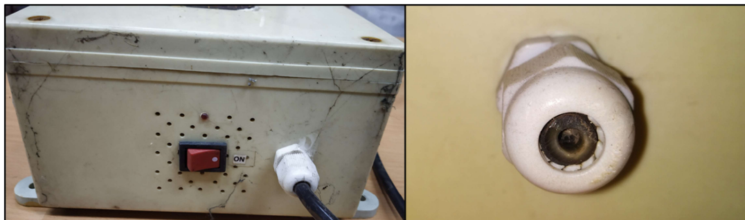
Figure 5.4: Spider webs outside a) and in the inlet b) of the Airveda low-cost sensor (AV_0027) installed at Nadampur. The images were captured on 20 December 2019 at the end of the field deployment at Nadampur.
