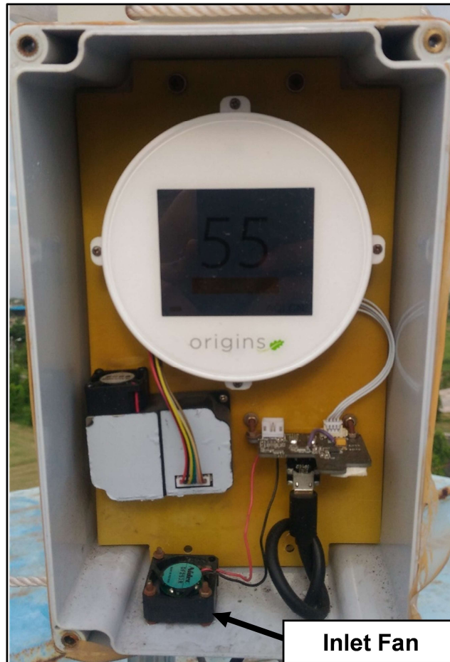
Figure 4.2: Figure showing the external casing, accessory inlet fan, and internal circuitry of the modified Laser Egg (LE) PM sensor.
