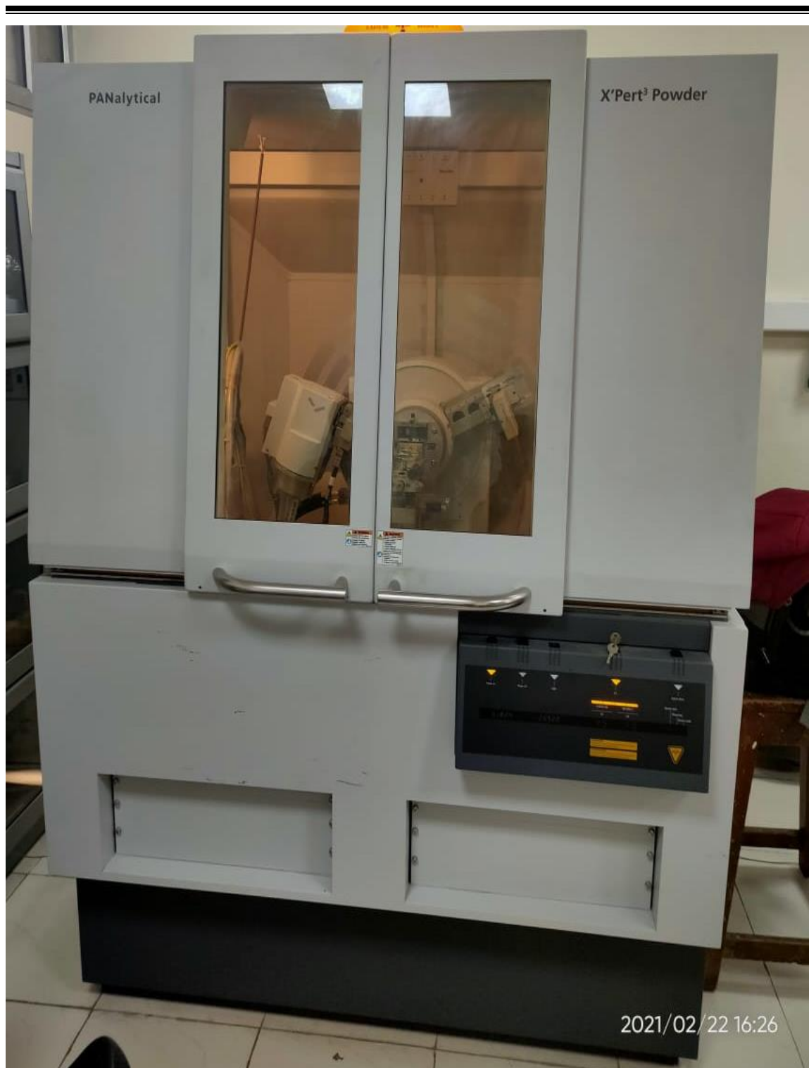
Figure 1.12. A typical view of grazing incident X-ray diffractometer.
