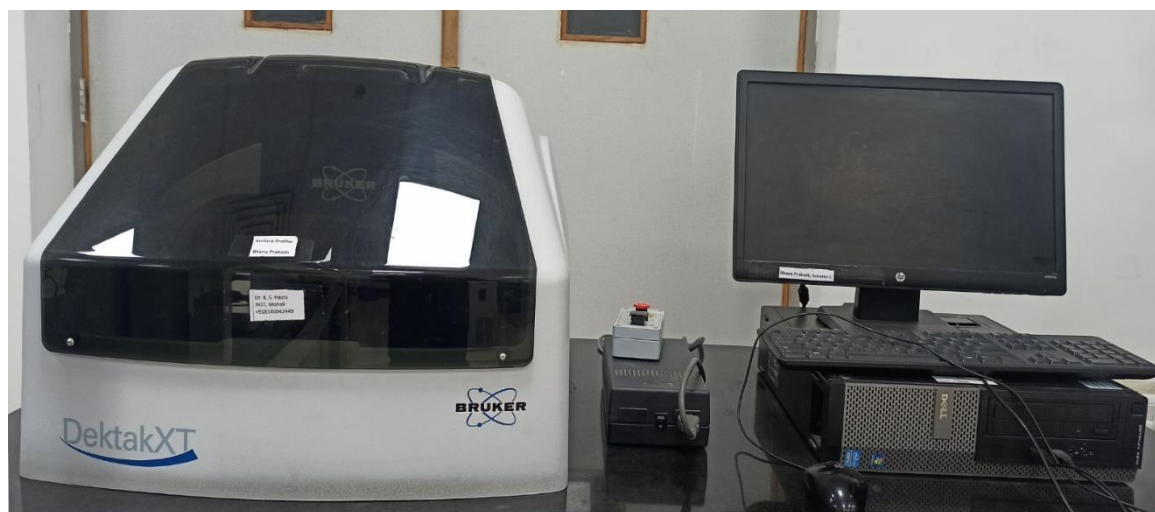
Figure 1.19. Typical view of the profilometer.
