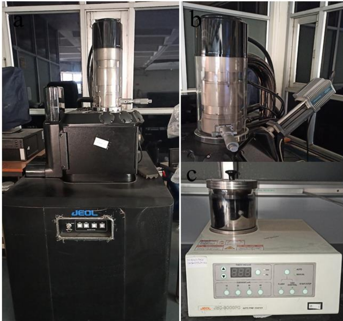
Figure 1.17. (a) A typical view of SEM column. (b) The EDX detector (backside of column). (c) Gold coater unit.
