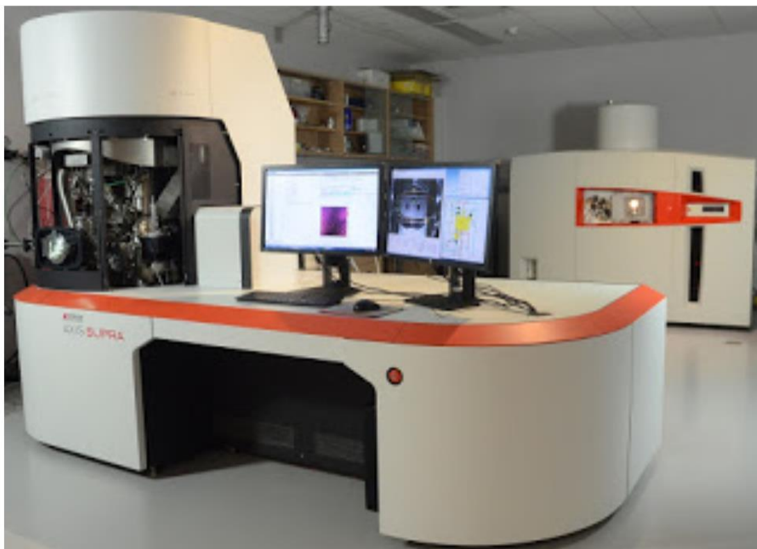
Figure 1.26. A typical XPS instrument.
