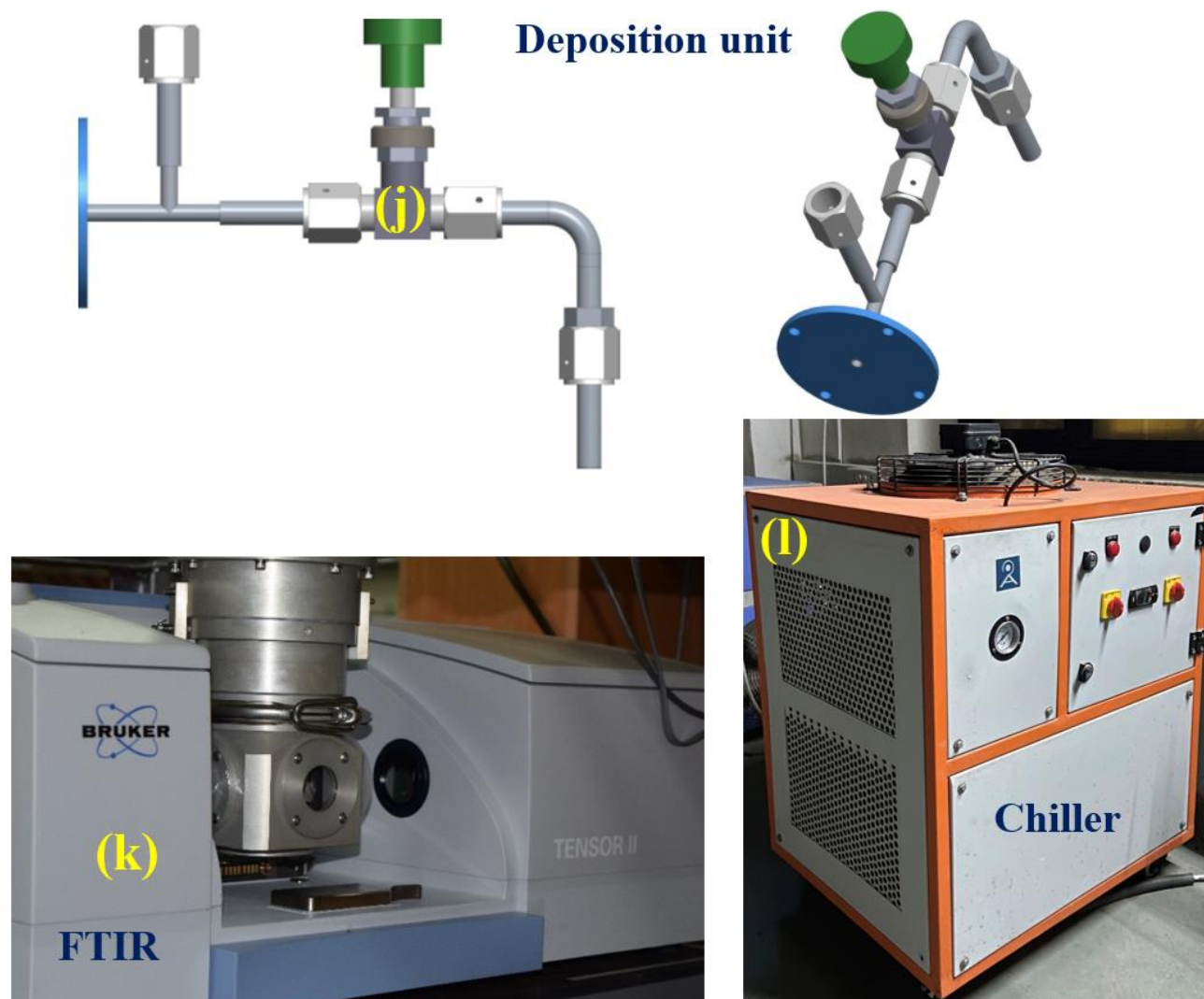
Figure 7.2 Remaining parts of matrix-isolation setup (j) designed deposition unit; (k) FTIR spectrometer; (l) chiller.
