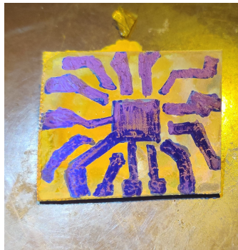
Figure 5: A PCB with sketched arms made for measuring resistance between the two plates of a thin film capacitor.
