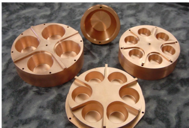
Figure 3.1: Crucible used to hold e-beam target. Structures with many buckets can hold multiple targets which can be changed as the crucible are rotated.
