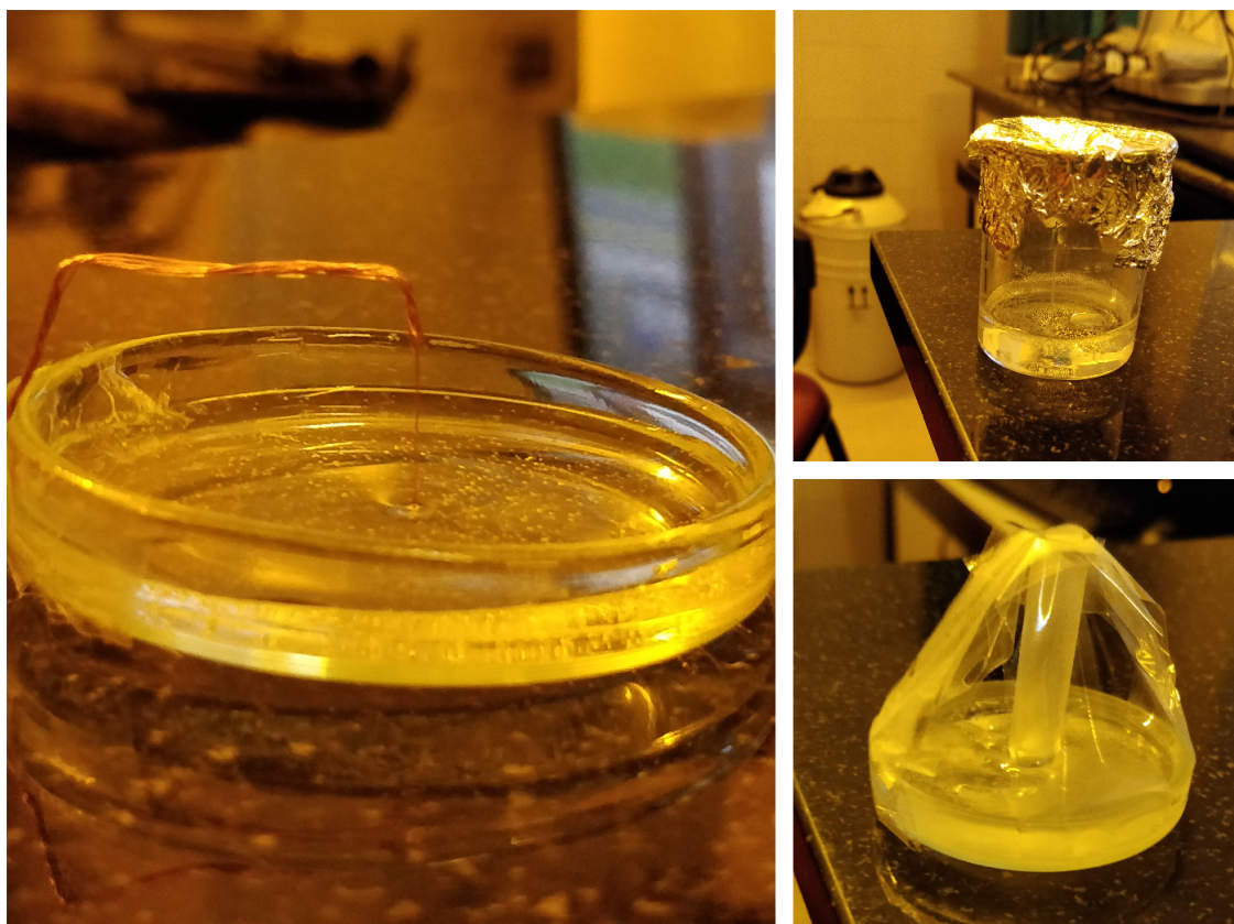
Figure 4.3: To reduce the diameter of the cylindrical hole, a wire was used as shown in figure on left. The 3/7 mixture was placed on magnetic stirrer using magnetic beads as shown in figure on top right. The bottom right figure shows the gel with a glass rod in the middle.
