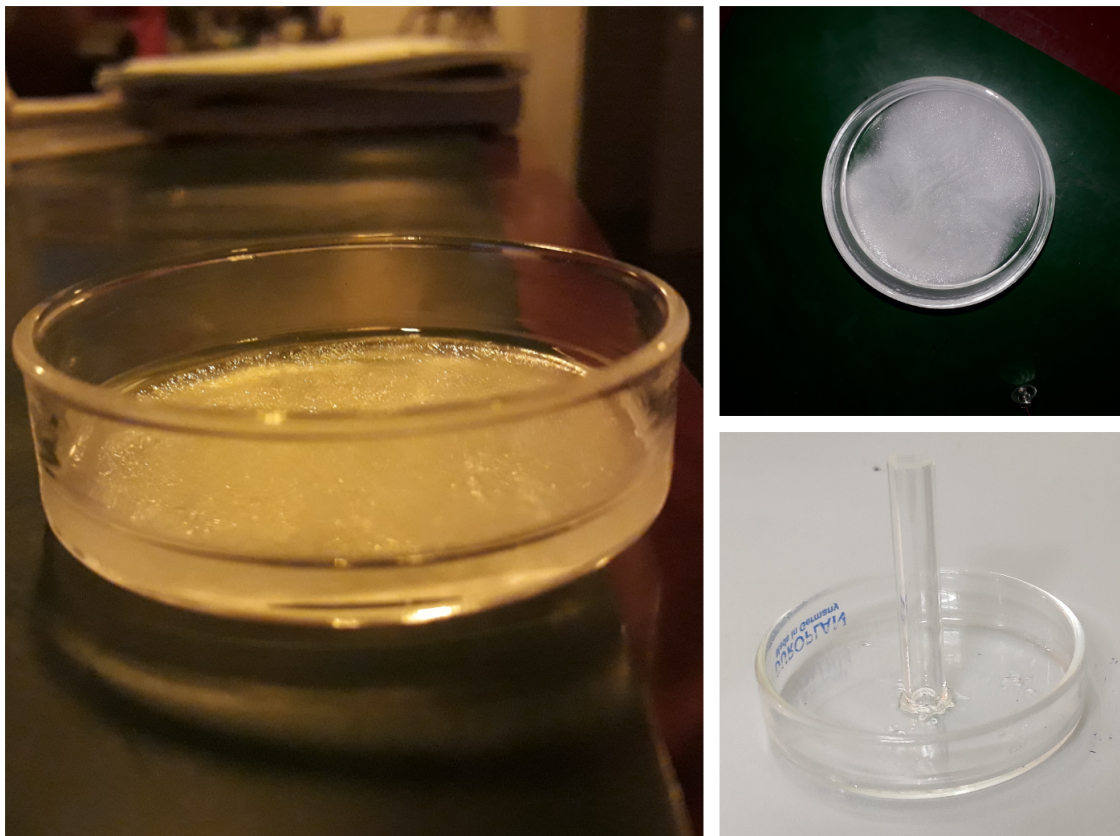
Figure 4.2: The three images here are the gels made around a glass cylinder. The cylinder was removed after gelation. The optical axis of the microscope was perpendicular to the cylinder axis and the tube was filled with an aqueous suspension of microspheres.
