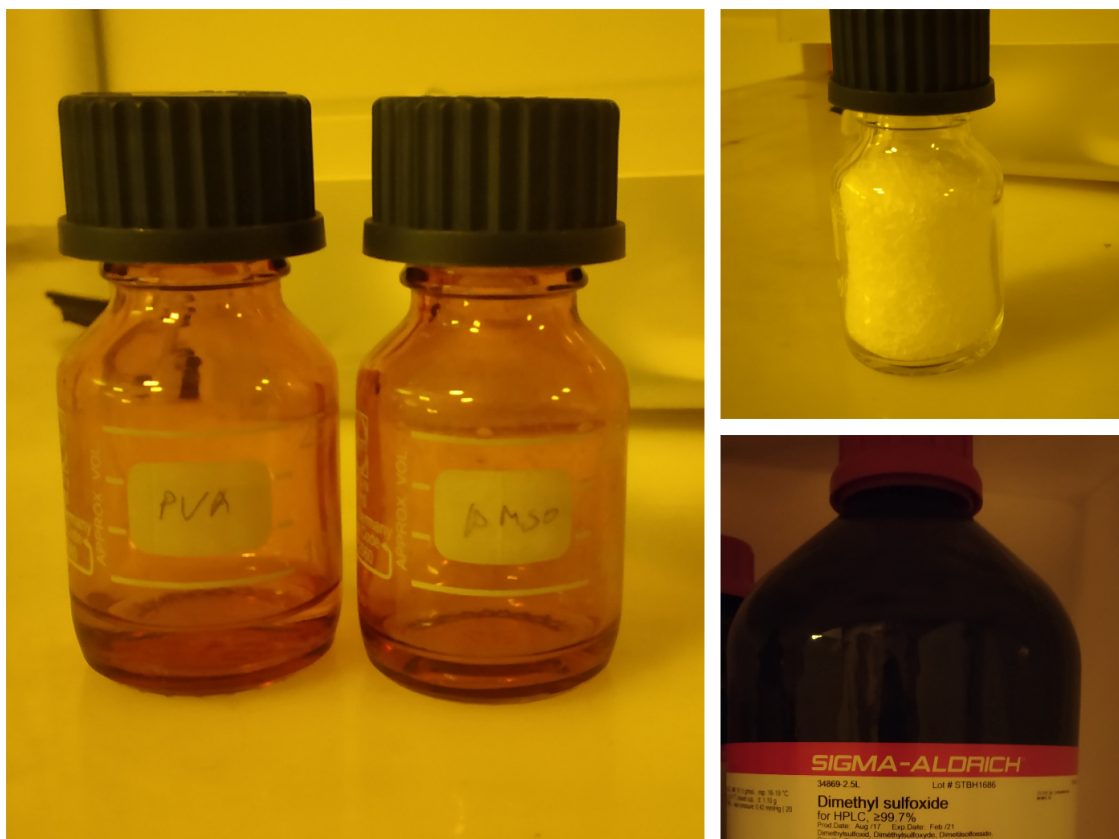
Figure 4.1: The top right figure shows Polyvinyl alcohol (PVA), which is readily soluble in water and was used to make PVA gel. The bottom right image shows DMSO used. The left image shows 10% PVA solution in water and 10% PVA solution in dimethyl sulfoxide (DMSO), which was mixed further in 3/7 ratio to make a cylindrical gel.
