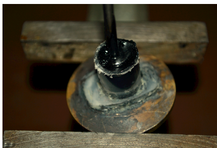
Figure 3.5: SS tube, first brazed, and then covered with stycast to the KF-25 blank, used to connect can with bellow, while testing leak using helium leak detector.
