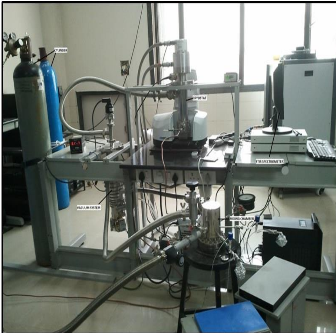
Fig 2.5: Matrix Isolation Spectroscopy setup in IISER-Mohali
