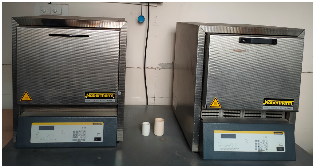
Figure 2.1: Two table top muffle furnaces used to give heat treatment in air.
