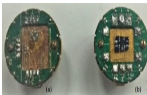
Figure 2.7: Sample mounted on a (a) DC resistivity and (b) AC resistivity puck.
