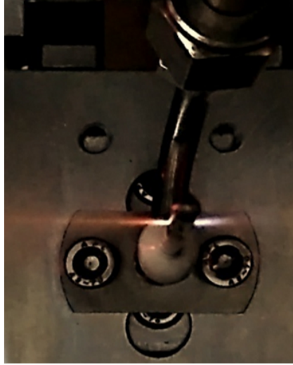
Figure 2.6: Ar gas filled capillary showing white light filamentation with XUV pulses generation.
