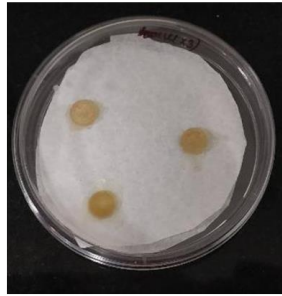
Fig 2.7 Digital Picture of ivory colored upconversion quartz coverslips. The coverslips were inserted at equal distance in button mushrooms for its exposure in solar simulator and laser irradiation
