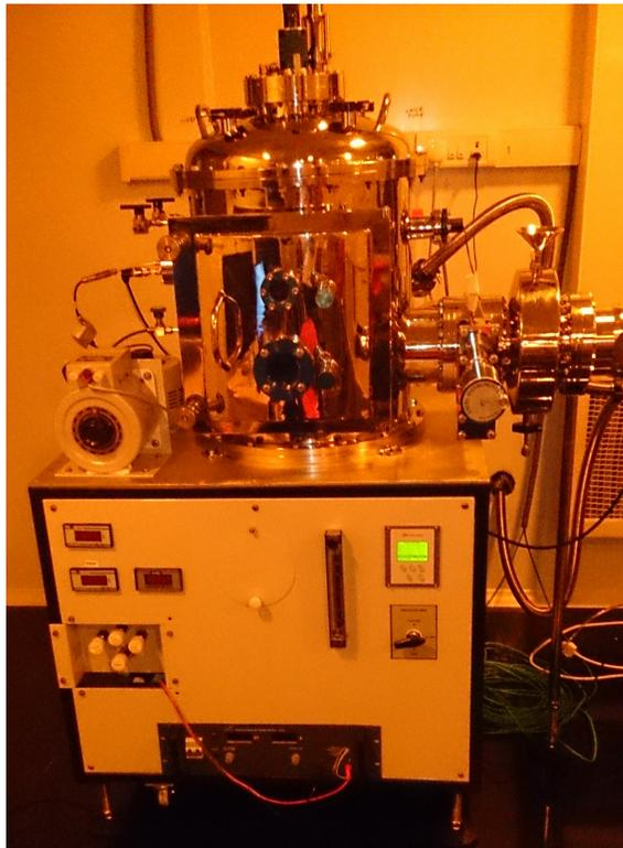
Figure A.5: Evaporation unit: This is used for evaporating different metals. This unit also has sputtering option
