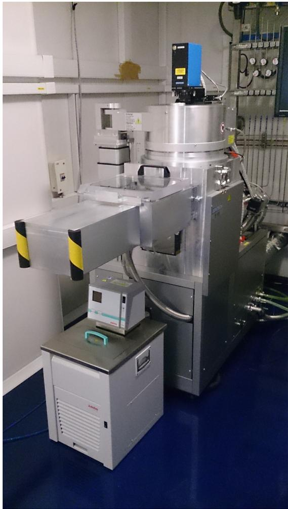
Figure A.6: Plasma Etcher: This is used for etching metals with the help of plasma.
