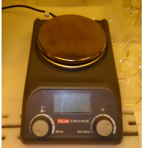
Figure A.3: Hot plate: This is used for baking LOR and PMMA after coating.
