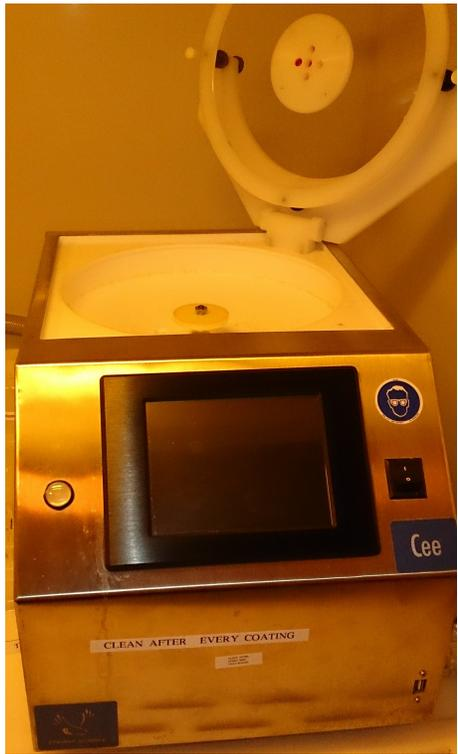
Figure A.2: Spin coater: This is used for coating substrate with LOR and PMMA.
