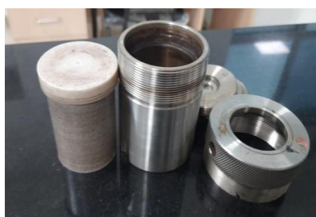
Fig 2.2: (a) Hydrothermal vessel (b) Details of steps involved in hydrothermal synthesis.
