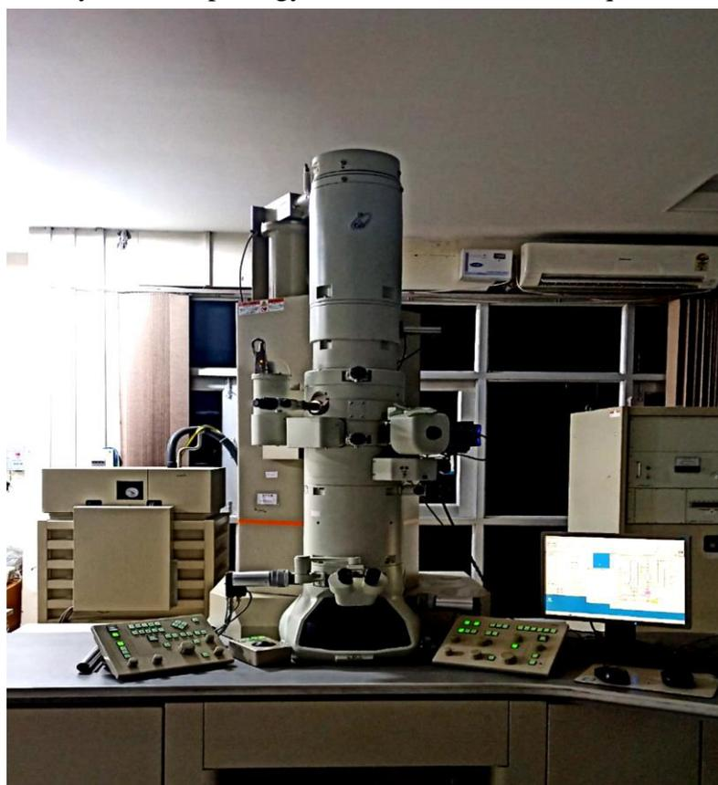
*Figure 2.7 Digital image of transmission electron microscopy.*
