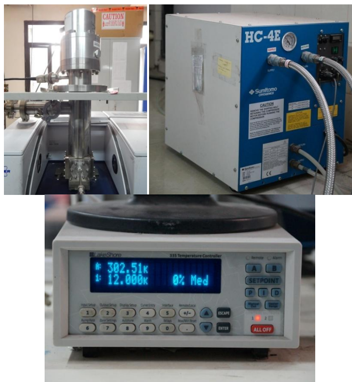
Fig. 2.6: (From L-R) a) The cryostat b) The He Compressor c) Temperature control unit
