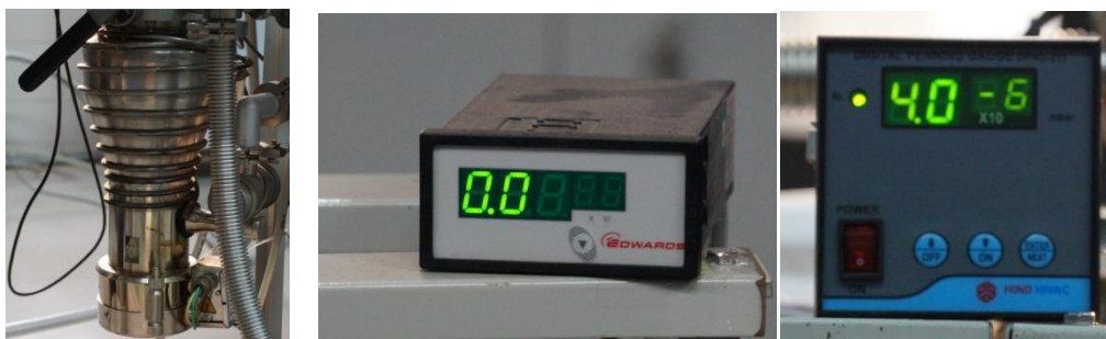
Fig. 2.7: (L-R) Diffusion pump, Penning Gauge and Pirani Gauge
