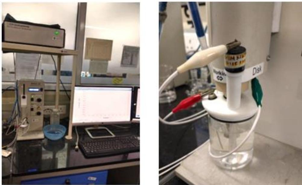
*Figure 13.* CHI760E electrochemical workstation for all electrochemical measurements.
