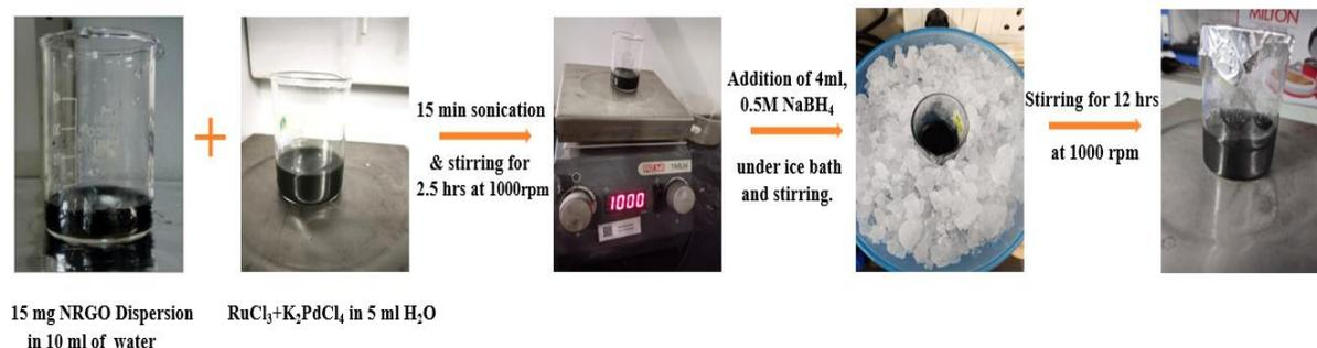
**Figure 17.** Schematic representation of reaction setup for synthesis of metal nanoparticles composites on NrGO.
