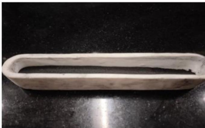
**Figure 15.** Nitrogen-doped reduced graphene oxide (NrGO) in Alumina boat
